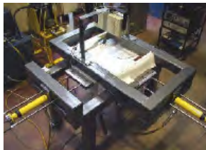
Fig. 7: Biaxial test rig (Bridgens et al., 2004)
