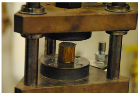
Figure 19: Smooth sugarcane specimen about to undergo compression test
