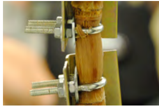
Figure 25: Side view of sugarcane specimen undergoing tension test
