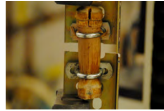
Figure 26: Front view of sugarcane specimen undergoing tension test
