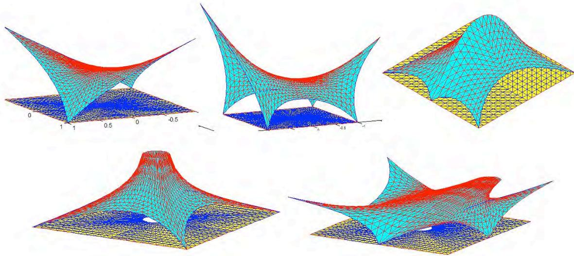
Figure 2: Viable configurations generated through the imposition of different sets of nodal displacements to the same plane squared reference mesh, with and without a hole.
