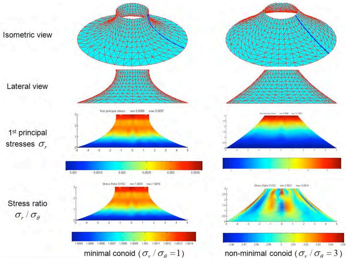
Figure 6. Comparison between minimal and non-minimal conoids.
