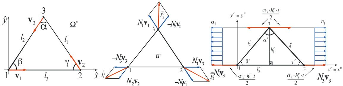
Figure 1. (a) Unit vectors  $\mathbf{v}_i$ ,  $i = 1, 2, 3$ , along the element edges; (b) internal nodal forces  $\mathbf{p}_i$ , decomposed into natural forces  $N_i \mathbf{v}_i$ ; (c) determination of natural force  $N_3$ .
