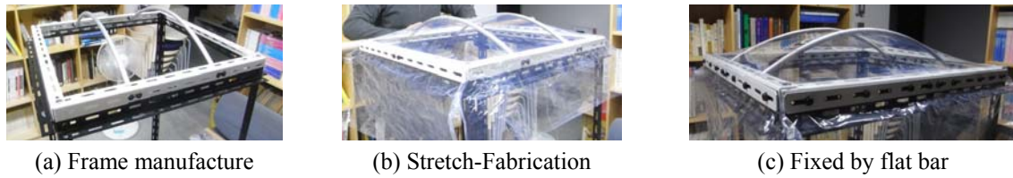
Figure 5: Manufacturing flow process
