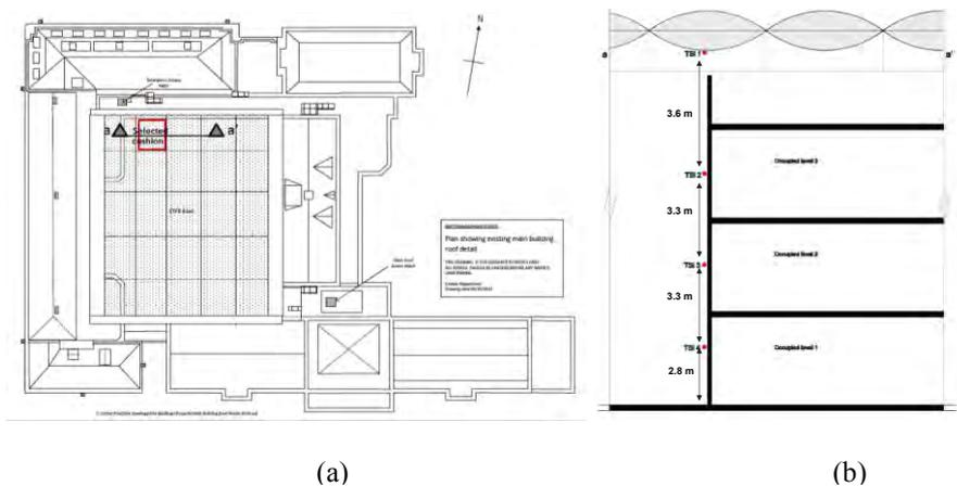
Figure 2: (a) Plan (nts) showing ETFE cushion roof and location of the monitored cushion, outlined in red (Drawing courtesy of Maber Architects, Nottingham), (b) Section showing vertical location of temperature sensors (Drawing: Sabrina Afrin)
