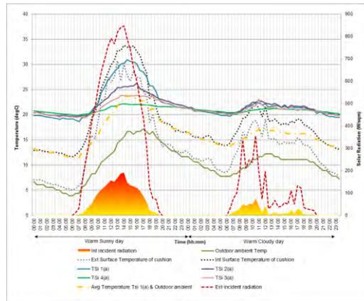
Figure 3: Typical thermal behaviour of the atrium during two consecutive days (one warm sunny and one cloudy) in April 2014
