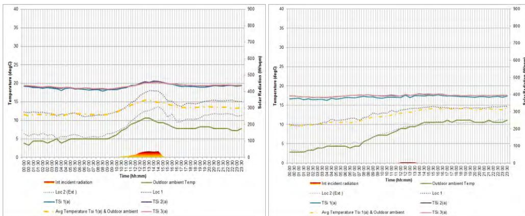
Figure 4: Typical thermal behaviour of the atrium during cold sunny (left) and cold cloudy (right) days in December 2013
