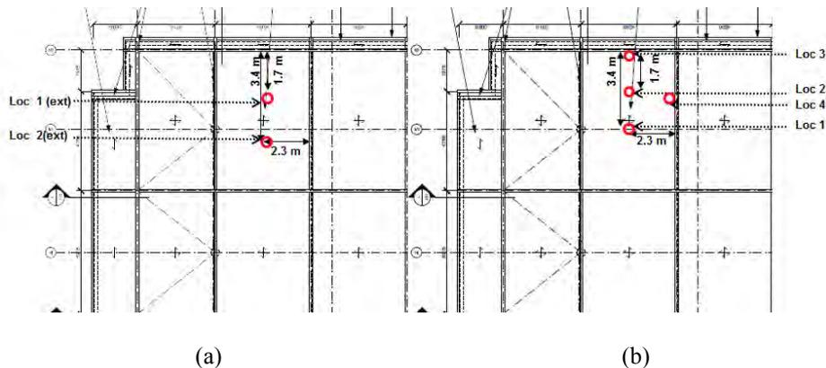
Figure 3: Plan (nts) showing ETFE cushion selected for monitoring and location of temperature sensors outlined in red (Drawing courtesy of Architen Landrell, Chepstow), (a) location of temperature sensors attached on external surface (b) location of temperature sensors attached on internal surface
