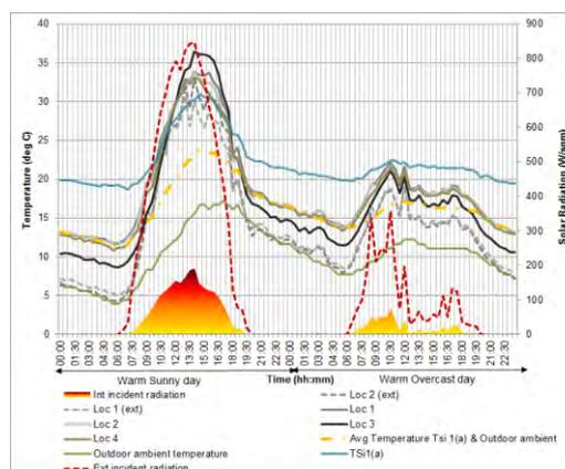
Figure 5: Typical thermal behaviour of the ETFE cushion during consecutive warm sunny and cloudy days in April 2014.
