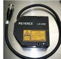
Figure 5: Three-dimensional photographic measurement system Figure 6: Laser displacement sensor
