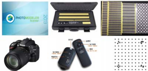
Figure 5: Three-dimensional photographic measurement system Figure 6: Laser displacement sensor
