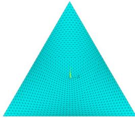
Figure 3: Meshing figure of ETFE cushion
